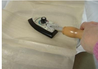
Figure 6—Pressing Fusible GlitterFlex Ultra while in hoop.
